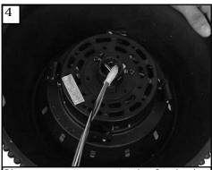
Place upper cover onto the fan body.
